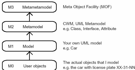
**Figure 3. Four-layered architecture (from [4])**
