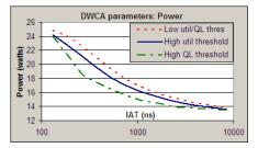
Fig 5. Power Consumption: Sensitivity to Utilization & QL Threshold
