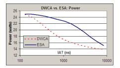
Fig 1. Power Consumption: Link Width & Power-state Controls
