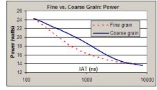
Fig 3. Power Consumption: Fine vs. Coarse Grain Width Control
