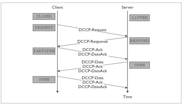
Figure 2. Datagram Congestion Control Protocol connection establishment. DCCP uses a three-way handshake to establish a connection.
