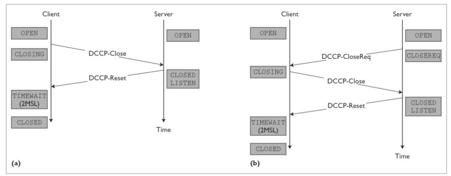
Figure 4. Datagram Congestion Control Protocol connection termination. DCCP uses two- or three-way handshakes to terminate a connection.
