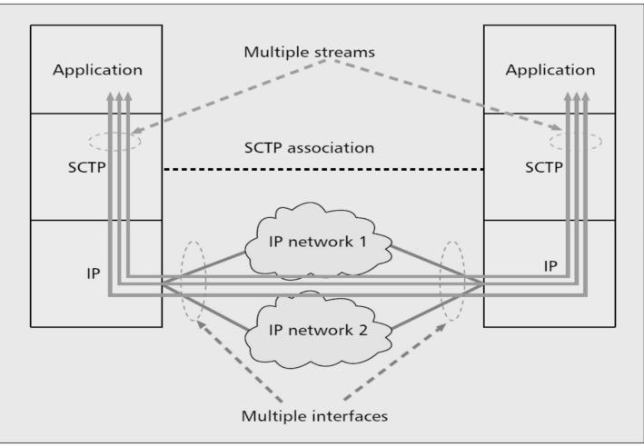
**Figure 1** A schematic view of an SCTP association
