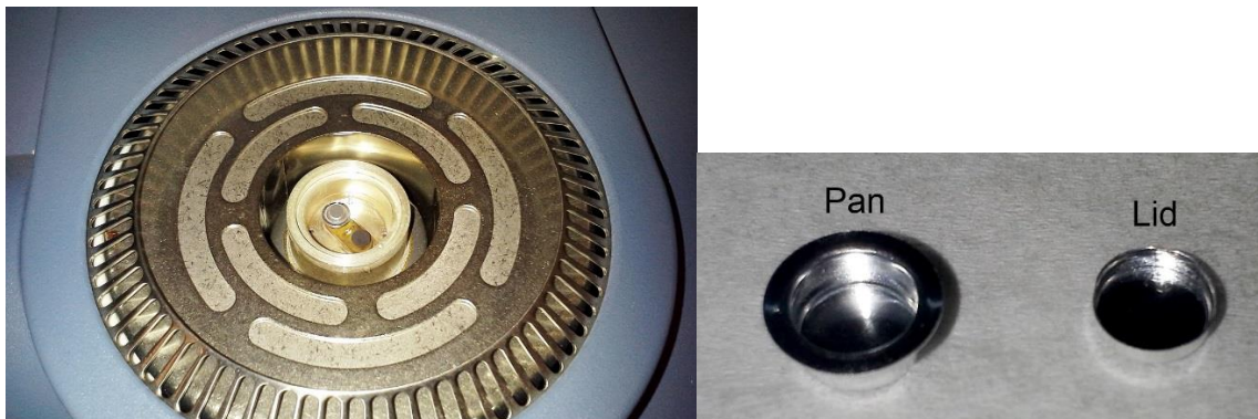
Fig. 7 DSC furnace (left) and sample pan + lid (right)
