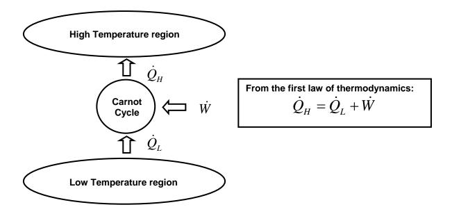
From the definition of Coefficient of Performance (COP), we find for the Carnot refrigeration cycle:
