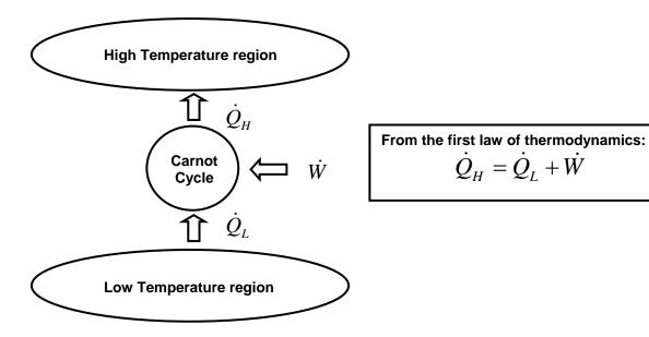
From the definition of Coefficient of Performance (COP), we find for the Carnot refrigeration cycle:
