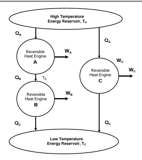
If we consider the Carnot cycle above, since a control volume could be drawn about engines A & B together, they may be considered as a single reversible engine. The efficiency of Engine A&B must be the same as that of Engine C since both are reversible. Also
