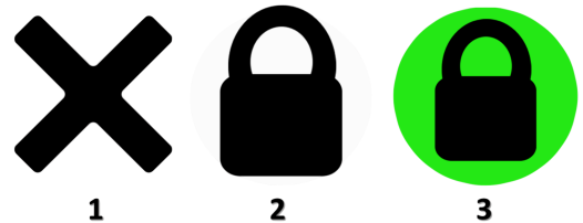
Figure 1: SafeKeeper browser addon icons: the first one indicates that SafeKeeper is unavailable on the website, or that the attestation protocol has failed; the second icon shows that SafeKeeper is supported and that a secure channel has been established; and the third icon is used when SafeKeeper is highlighting the protected input fields (see Section 3).
