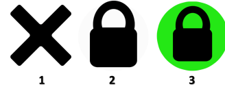
Figure 3: SafeKeeper browser addon icons: (1) SafeKeeper is unavailable on the website, or the attestation protocol has failed; (2) SafeKeeper is supported and a secure channel has been established; (3) SafeKeeper is highlighting the protected input fields (see Section 5.2.2).
