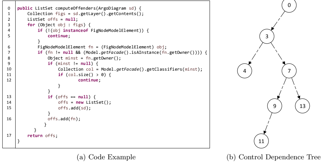
Figure 6: Code example and corresponding Control Dependence Tree
