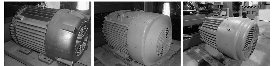
25, 60, and 100 hp induction motors tested using the proposed techniques.
