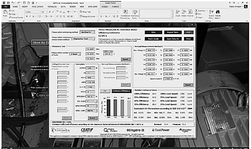
The developed software shows testing results of a 150 hp machine.
