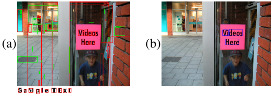
Figure 6: Clustering of CCs. (a) Text and non-text CCs identification. (b) Merging text CCs to generate the final result.
