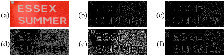
Figure 3: Edge detection using different methods. (a) Original Image. (b) Sobel edges. (c) Prewitt edges. (d) Canny edges. (e) Wavelet-based edges. (f) Bandlet-based edges.
