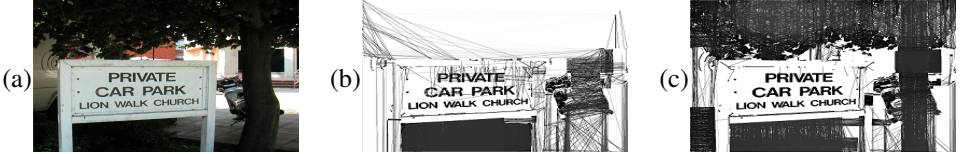
Figure 5: Stroke width transform of a sample image. (a) Original Image. (b) SWT output using bandlet-based edges. (c) SWT output using Canny edges.
