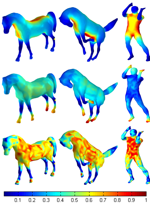
Fig. 5 Normalized \chi^2 -distance between a reference point (yellow colored on the horse's back left leg) and other surface points using different signatures. Top row : heat kernel. Middle row : wave kernel. Bottom row : cubic spline wavelet kernel with R = 2
