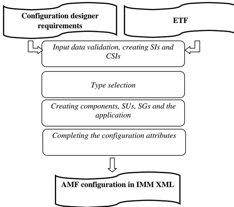
**Fig. 2.** Main steps for configuration generation.
