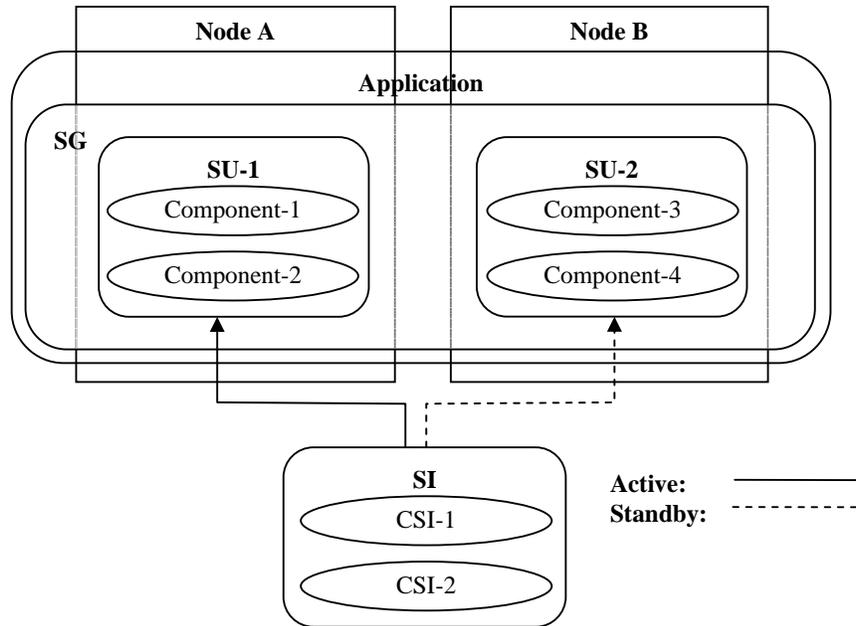
**Fig. 1.** Example of configuration of AMF entities.
