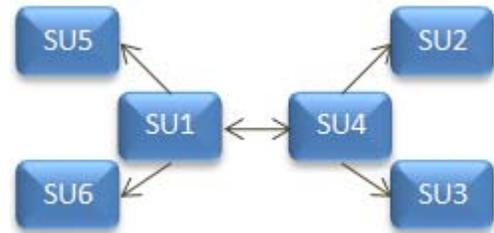
**Figure 2. The SU backup graph using the round robin algorithm.**
