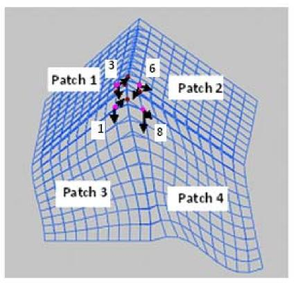
The construction of the NURB patch used to fill in the hole between four stitched patches with C1 continuity smooth transition
