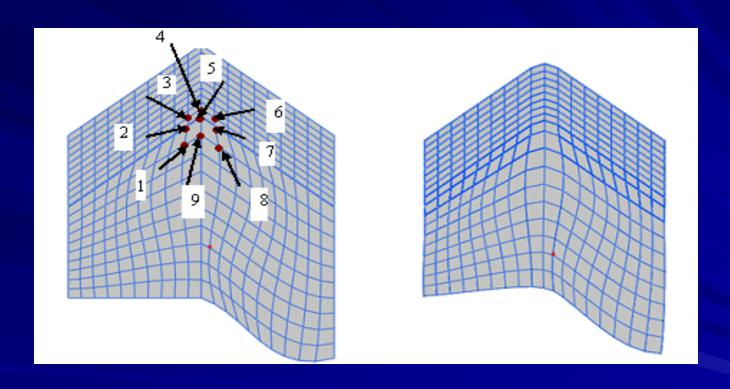
Four stitched patches before C1 and after C1connection.
