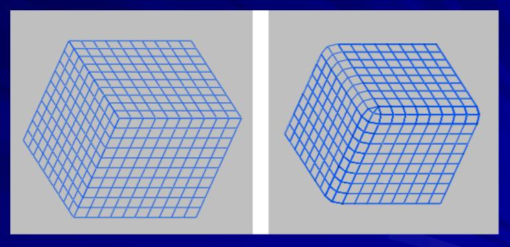
Three stitched patches before C1 and after C1connection.
