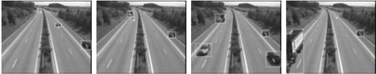
Figure 3. Tracking results of the sequence ‘Highway’. To show the reliability of the tracking algorithm only one in every five images has been used. This shows, for example, that the proposed method can track objects that move fast.
