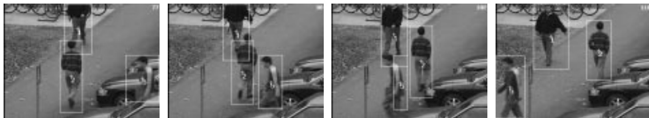
Figure 5. Tracking results of the ‘Survey’ sequence. Each object is marked by an ID-number and enclosed in its minimum bounding box. Despite the multi-object occlusion, light changes, and reflections, the algorithm stays stable. Note how the method recovered properly after the static traffic sign.
