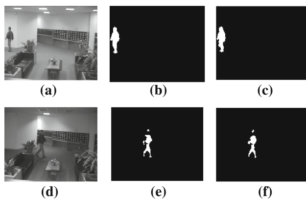
Fig. 20 Proposed FPGA implementation comparison to the software counterpart. Top row is frame 387 of the Switching Light Off video sequence and bottom row is frame 641 of the same video sequence after the light is switched off. First column is original I(n) , and second and third columns are binary B(n) frames with software and the proposed hardware implementation, respectively
