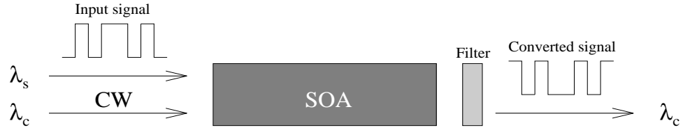
Figure 7: A wavelength converter based on XGM in an SOA.
