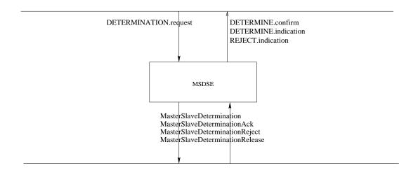
Figure 21: the Primitives among the MSDSE process, the MSDSE User, and its Peer Entity
