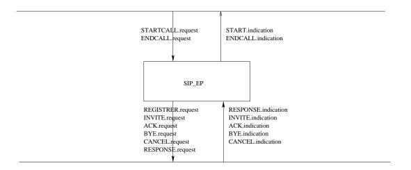
Figure 38: the Primitives between the CommandController process and the CommandController user, and its peer entity
