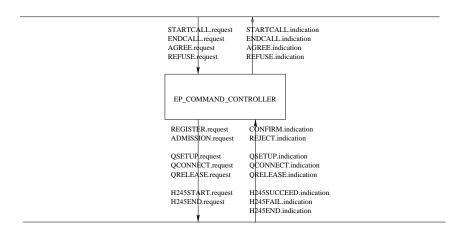
Figure 35: the Primitives between the EPController and the EPController User, and its Peer Entity
