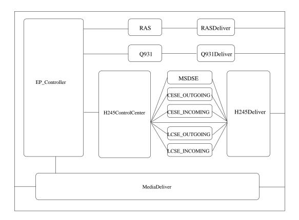
Figure 33: the Internal Structure of H323 Endpoint Block
