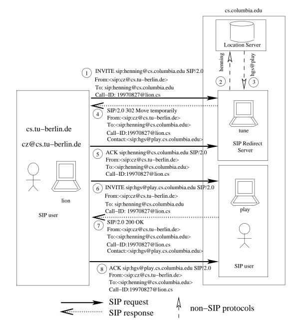
Figure 7: Protocol Exchange for SIP Redirect Server [3]
