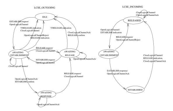
Figure 26: the Finite State Machine of outgoing LCSE process and incoming LCSE process
