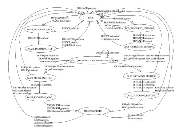
Figure 28: the Finite State Machine of H245ControlCenter Process
