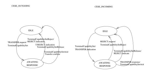
Figure 24: the Finite State Machine of outgoing CESE process and incoming CESE process
