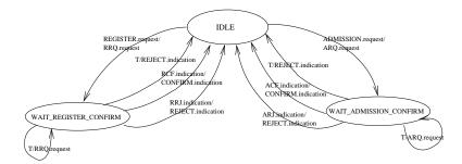
Figure 30: the Finite State Machine of RAS Process
