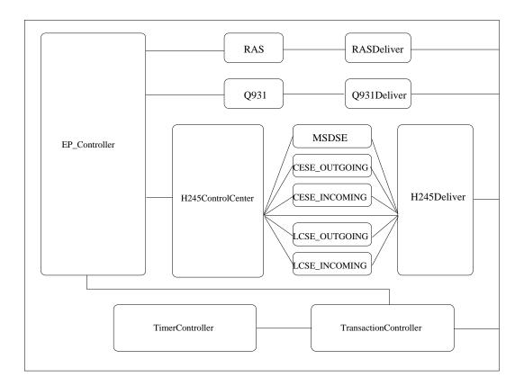
Figure 40: the Internal Structure of SIP-H.323 IWF Block
