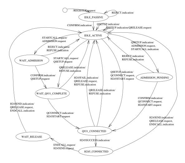
Figure 36: the Finite State Machine of EPController in H.323 EP
