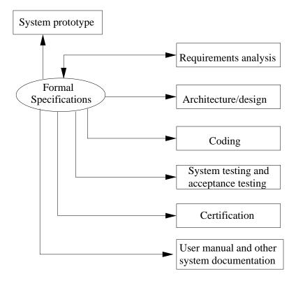
Figure 10: Using Formal Specifications in Different Stages of Development Life Cycle [10]
