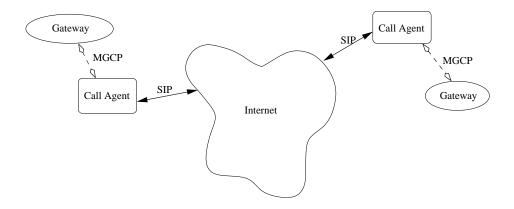
Figure 8: A System using MGCP and SIP
