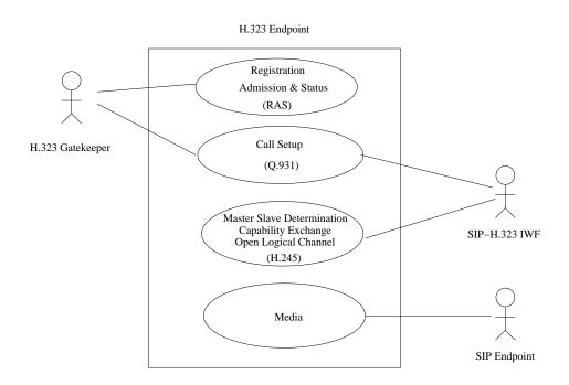
Figure 11: H.323 Endpoint Use Case Diagram
