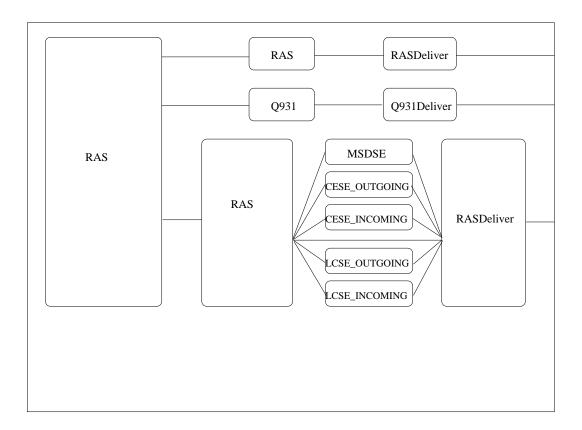
Figure 19: the Internal Structure of H.323 EP Super Block Type
