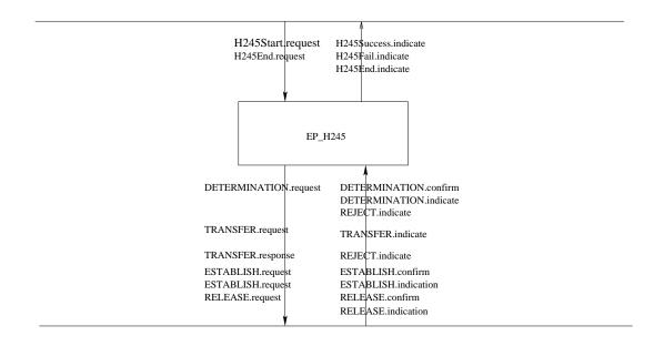
Figure 27: the Primitives between the H245ControlCenter and H245ControlCenter user, and its peer entity
