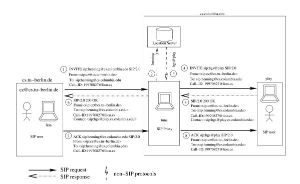
Figure 6: Protocol Exchange for SIP Proxy Server [3]
