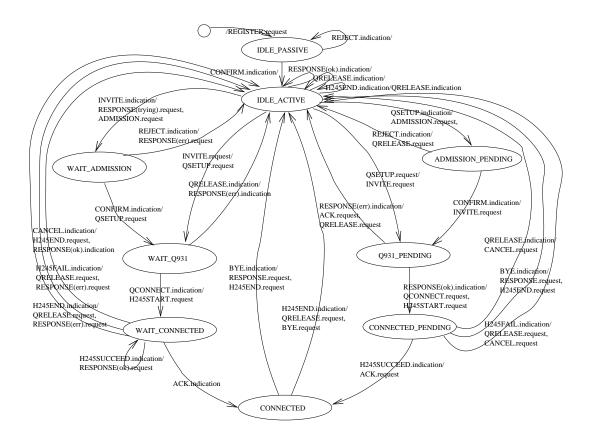
Figure 43: the Finite State Machine of EP\_Controller in IWF
