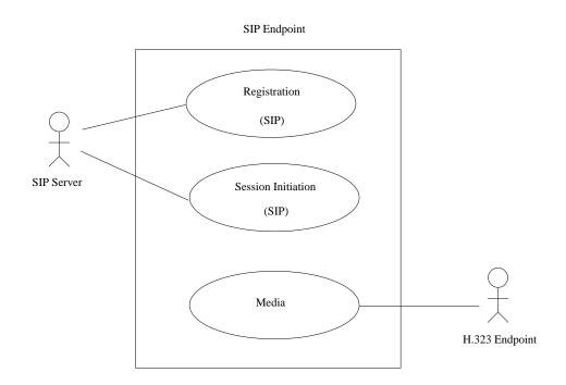
Figure 12: SIP Endpoint Use Case Diagram
