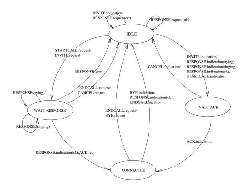
Figure 39: the Finite State Machine of the CommandController process
