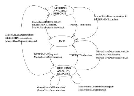
Figure 22: the Finite State Machine of MSDSE process
