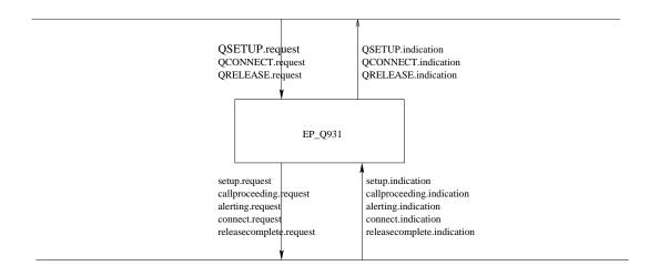
Figure 31: the Primitives among the Q931, the Q931 User, and its Peer Entity
