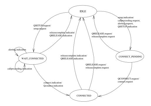
Figure 32: the Finite State Machine of Q931 Process
