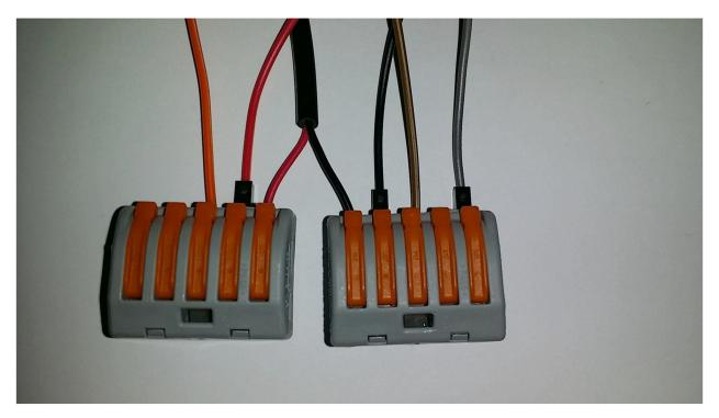
7. Connect the male end of the grey wire to the lever nut block as follows.
