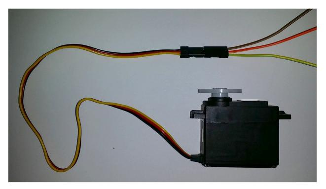
6. Connect the stripped ends of the brown and orange wires into the lever nut blocks as follows. Note that the female end of the yellow wire will be connected to the Arduino later on.
