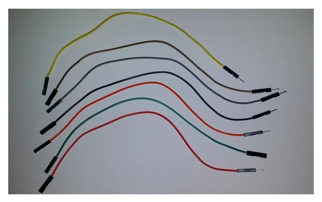
3. Remove the female connectors/ends from the brown and orange wires. Note if you have male / male brown and orange jumper wires then you don't require this step – just substitute the male / male jumpers for the stripped wires. Then strip the ends (see first picture below), bend back the ends (i.e. bend the stripped ends in half), and twist the ends as shown in the second picture.
