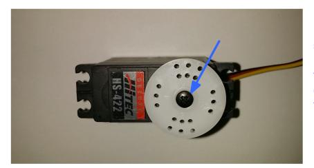
Note: After the front screw is removed then remove the back screws (see step #8) while holding the front of the case together with the back of the case to prevent the gears from falling out.
