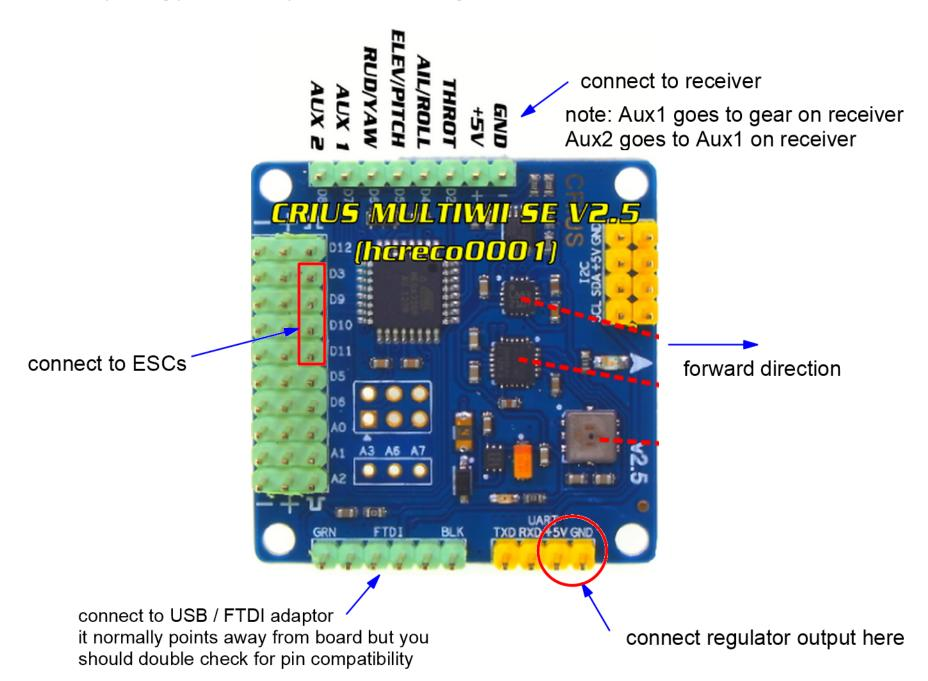
Connecting a Flip MultiWii 2.5/2.6 board is basically the same as the Flip 1.5 except the pins are in different locations and the forward direction is different. The following diagram shows the corresponding pins to the Flip 1.5 connection diagram above and the forward direction.
