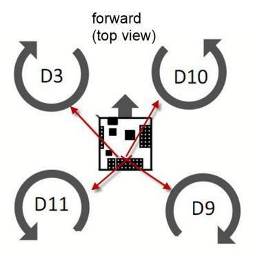
The motor directions (top view) for a guad configuration are also indicated in the diagram. Note the propellor directions should be selected so that they push air down with the corresponding motor directions.
