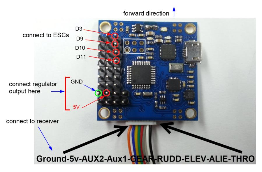
note: Aux1 goes to gear on receiver Aux2 goes to Aux1 on receiver
