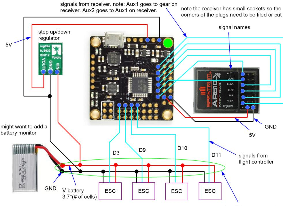
note: some ESCs have two inputs -- a signal and a GND. The GND can be connected to the GND of the flight controller or battery
