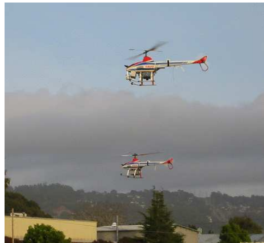
Fig. 1. Flight experiment with multiple autonomous helicopters (Photo Courtesy of Hoam Chung)
