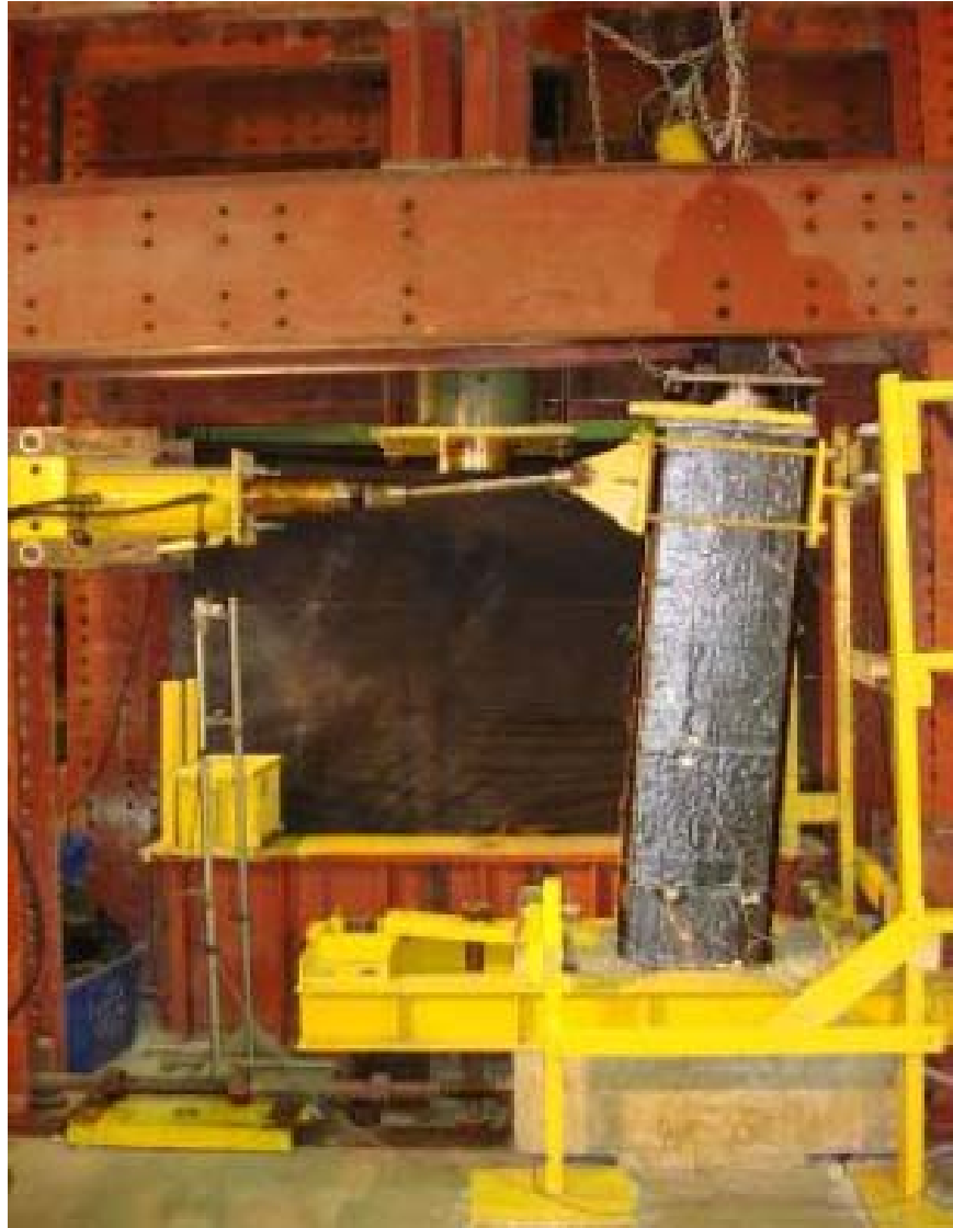
Rehabilitated RM column under axial and lateral loads
