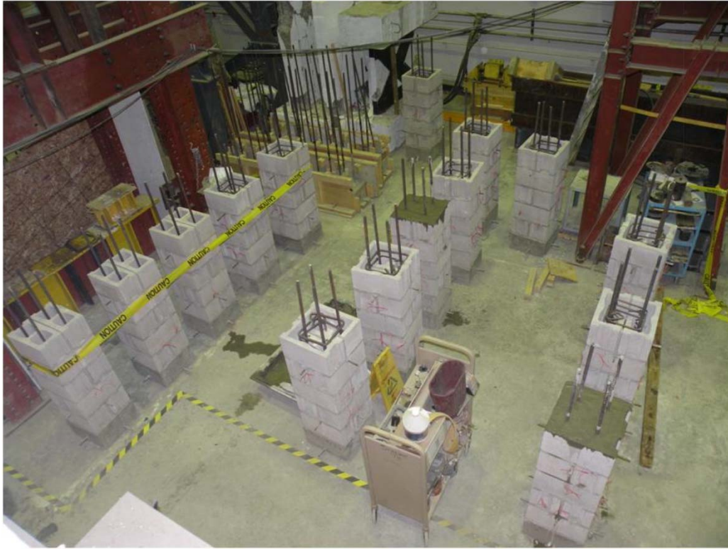
Construction of full-scale reinforced concrete block boundary elements
