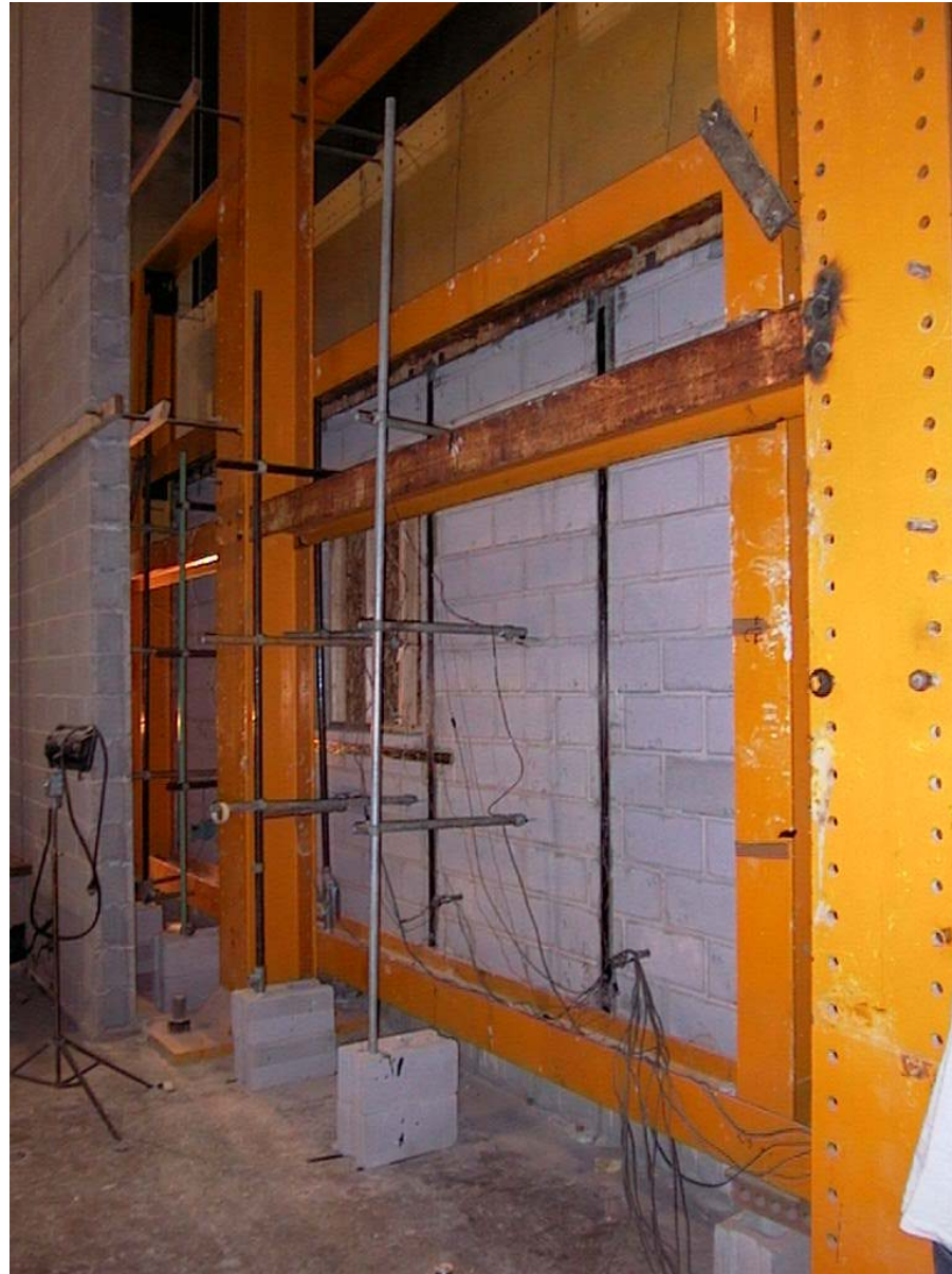
Strengthened Wall in the test setup
