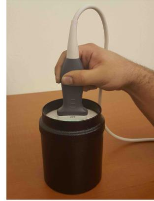
Fig. 2. Setup for phantom studies: The probe is hand-held during data collection from a CIRS elastography phantom. An excitation with period of  $160\mu\text{s}$  at the focal depth of 20mm is applied as ARF and a set of 80 RF frames were acquired to monitor the shear-wave.
