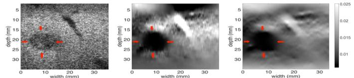
Fig. 2 In-vivo data: BMODE image, DPAM strain, GTDE strain.
