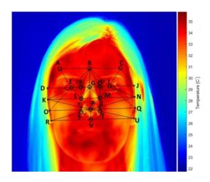
A thermal image sample recorded during a laboratory study which shows the facial landmarks tracking results.
