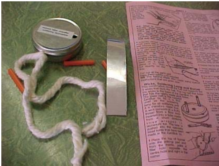
Making the burner is very simple as the burner fuel tank is already punched for the burner tubes. There are 3 holes, but 2 are covered with a sticker. The orange drinking straw tubes are covered with rectangles of the heavy aluminum foil. The mop string has 4 sub strings, but only 3 will fit so one must be removed.
