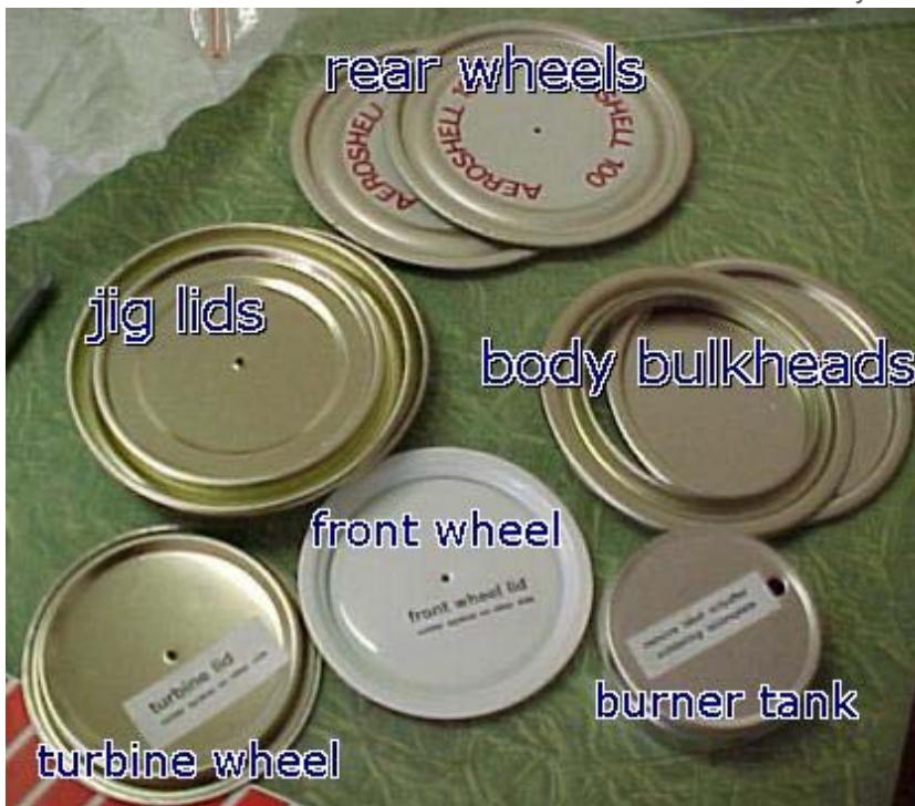
The collection of lids used for wheels etc. When I first unpacked it all I was confused by the 2 extra lids which later turned out to be for the wheel soldering jig. This is made by wrapping a strip of steel around the 2 lids to form a cylinder. This is held together by a sticky label. One of the axles is placed through the holes, the wheel on top, then the spoke plate on top of that. The cylinder ensures that the axle is perpendicular to the wheel surface, so that when the spoke plate is soldered on the wheel does not wobble. Well that's the theory anyway. I managed to get the turbine to wobble and will have to redo it sometime to get it to balance better.
