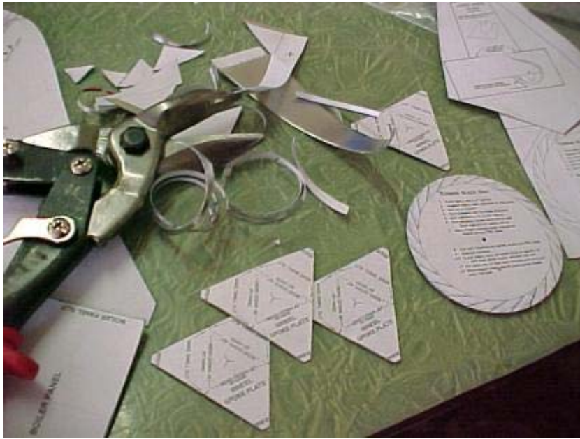
After a pleasant hour's cutting with my geared tin snips I have a pile of scraps and 4 spoke plates (the triangular bits), the turbine blade wheel, and the body plate at left.
