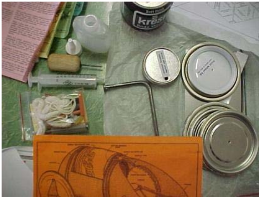
More unpacked parts. Top left is the water filling bottle, below that the awl made from a bicycle spoke and section of dowel, the fuel filling syringe, the smaller bag of parts, to the right of the the big bent nail for enlarging the burner holes, the burner fuel tank.
