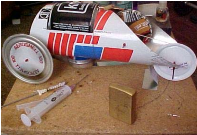
The completed car just before the first run. The wheels are fitted and held in place by slipping short bits of rubber tube over the axles. The burner is held in place by a long strip of metal that hooks in just behind the front wheel and hooks over the rear axle. This can be removed so that the wicks can be serviced.
