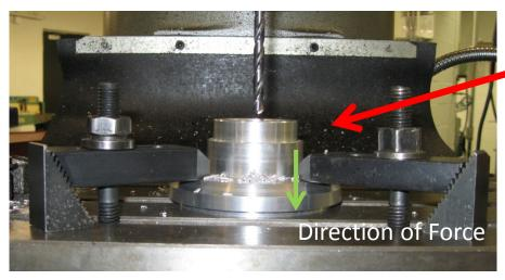
Metal-on-metal on-metal. It can be seen that clamping force is transferred directly into the table.
