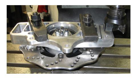
If necessary, entire assemblies can be clamped to a milling table, to do certain processes in order to finish assemblies. Although not ideal, these actions are performed in certain cases when it may be very difficult and/or expensive to dismantle the assembly.
