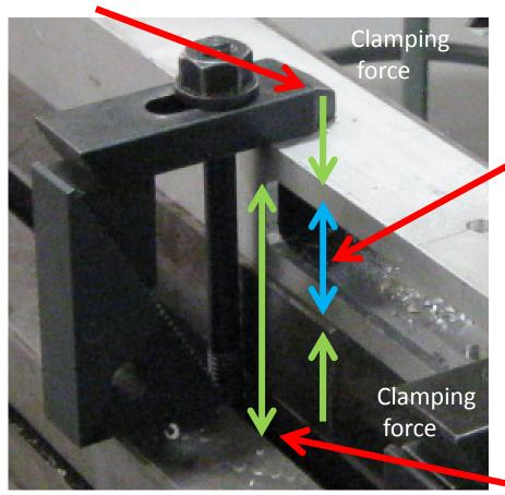
Support Structure. A rigid piece of material that fits the exact space (adjustable items, such as screw jacks are recommended here) would allow the clamping force to be properly transmitted to the table through the blue arrow (representing a support).
