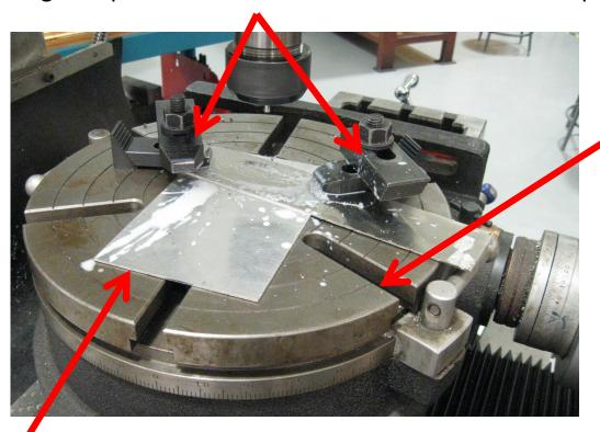
Rotary Table. This tool allows the work to move in polar directions. Set up time for this tool can be long, complicated, and difficult depending on required precision. Good design for manufacturability should minimize the use of this tool.
