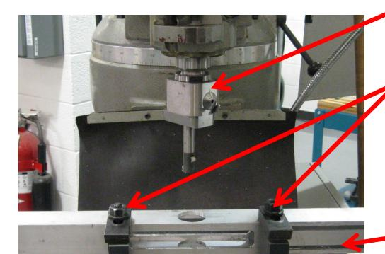
Boring Head use is time consuming. Try to use standard hole sizes to avoid using the boring head.
