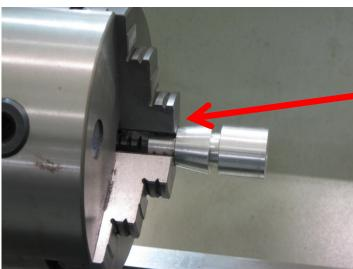
Standard 3 jaw chucks use 3 point of contact to secure tools or parts. Properly installed, the tool or part will rotate about the center of the chuck.
