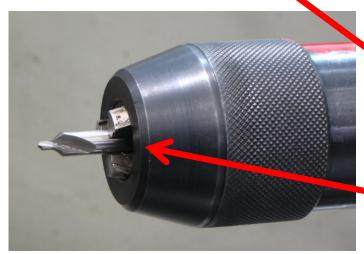
Drill chucks as well as other 3 jaw chucks clamp down onto tools with 3 points of contact.
