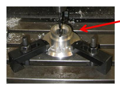
No Twist. The addition of the third clamp distributes the forces, minimizing distortion. Two clamps on opposing sides of the work will also work to stop twisting of work.
