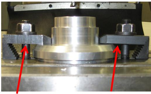
Metal-on-metal-on-metal. This setup does not have the clamping force directed onto the table surface directly.
