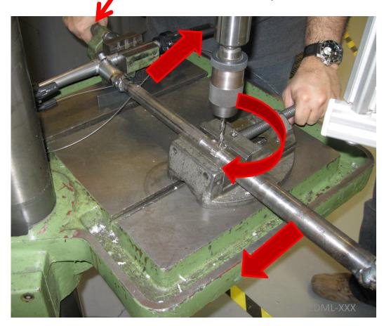
No Twist! In this setup, the operator is being used to resist the torque generated by the revolving cutter. If the drill were to bind (common on breakthrough), the operator would be struck and injured by the now-revolving work piece. This is unsafe practise! Use a fixed object like the column of the pedestal to resist cutting torque.
