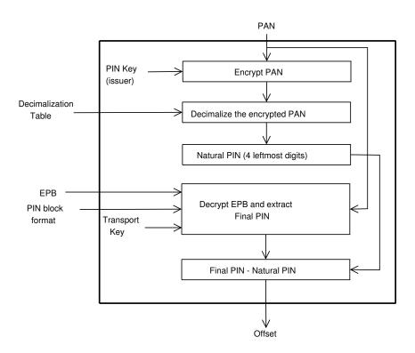
Figure 8.1: Offset calculation (adapted from [194])
