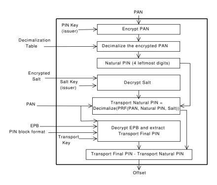
Figure 8.3: Salted-PIN verification for the IBM offset method
