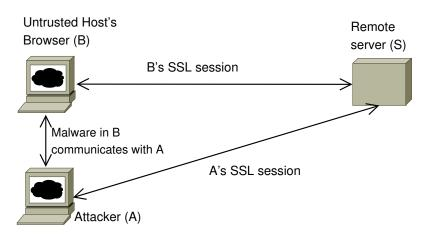
Figure 3.2: Setup for a parallel session attack
