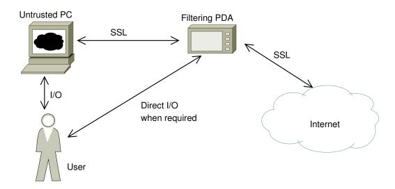
Figure 4.6: Guardian setup (adapted from [156])
