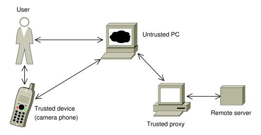
Figure 4.4: Camera-based authentication
