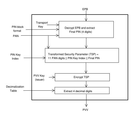
Figure 8.2: PVV calculation (adapted from [194], || denotes concatenation)
