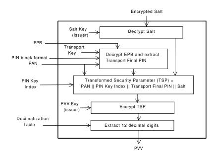
Figure 8.4: Salted-PIN verification for the VISA PVV method
