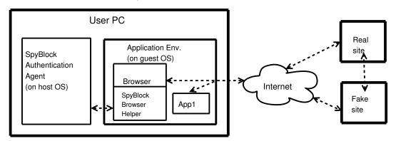
Figure 4.2: SpyBlock setup (adapted from [129])
