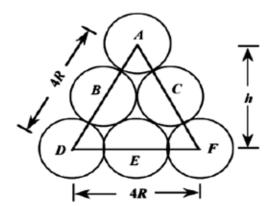
There are six atoms whose centers lie on this plane, which are labeled A through F. One-sixth of each of atoms A, D, and F are associated with this plane (yielding an equivalence of one-half atom), with one-half of each of atoms B, C, and E (or an equivalence of one and one-half atoms) for a total equivalence of two atoms. Now, the area of the triangle shown in the above figure is equal to one-half of the product of the base length and the height, h. If we consider half of the triangle, then
