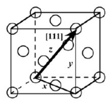
For this [111] direction, the vector shown passes through only the centers of the single atom at each of its ends, and, thus, there is the equivalence of 1 atom that is centered on the direction vector. The length of this direction vector is denoted by z in this figure, which is equal to
