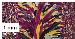
Nb-Hf-W plate with an electron beam weld
