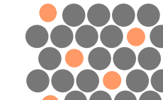
Substitutional solid soln. (e.g., Cu in Ni)
