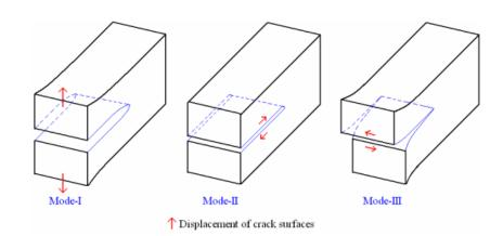
**Mode-I** is a tensile type of fracture, in this mode fracture the crack surfaces are displaced normal to themselves.
