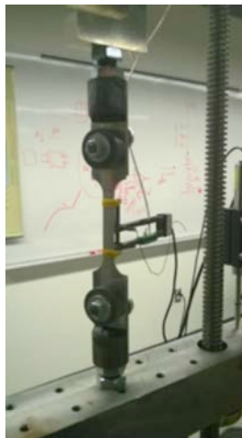
Figure 1.10: Mounting Tensile Sample
