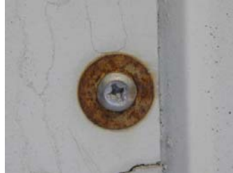
Stainless screw and cadmium plated steel washer
