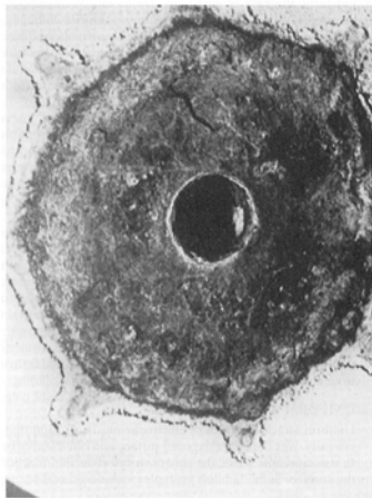
FIGURE 18.14 Galvanic corrosion of a magnesium shell that was cast around a steel core.
