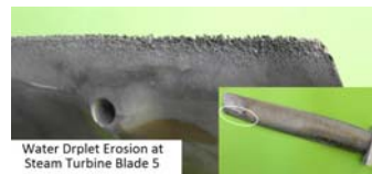
Alstom Steam Turbine, airfoil A. Uihlein, EPRI 2012
