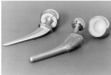
FIGURE 23.14 (Callister 5 th ed.) Photograph showing two artificial total hip replacement designs.
