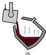
Charging pig iron
