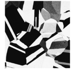
Grain growth after 10 min at 700°C
