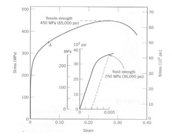
A cylindrical specimen of this alloy, 20 mm in diameter and 188 mm long, is to be pulled in tension. Calculate the stress (in MPa) necessary to cause a 0.0136 mm reduction in diameter. Assume a value of 0.34 for Poisson's ratio.
