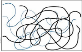
(a) Linear unbranched polymer: notice chains are not straight lines and not connected.
