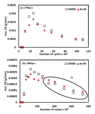
Figure 7: Inst. ER for As-M and UNSM airfoil samples at different impact speeds [9].
