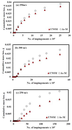
Figure 4: WDE curves of As-M versus UNSM flat samples at different impact
