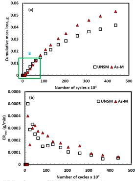
Figure 8: WDE performance of UNSM airfoil without edge treatment *versus* As-M at 300 m/s.
