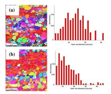
Figure 3: EBSD images of (a) untreated and (b) UNSM treated conditions.
