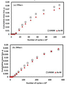
Figure 6: WDE curves of As-M and UNSM airfoil samples at different impact speeds [9].
