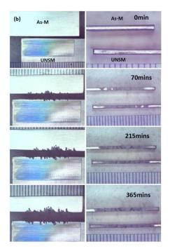
Figure 9: OM images showing (a) the untreated airfoil edge and (b) the erosion evolution and progression on As-M and UNSM (with untreated edge) airfoil samples at 300 m/s.
