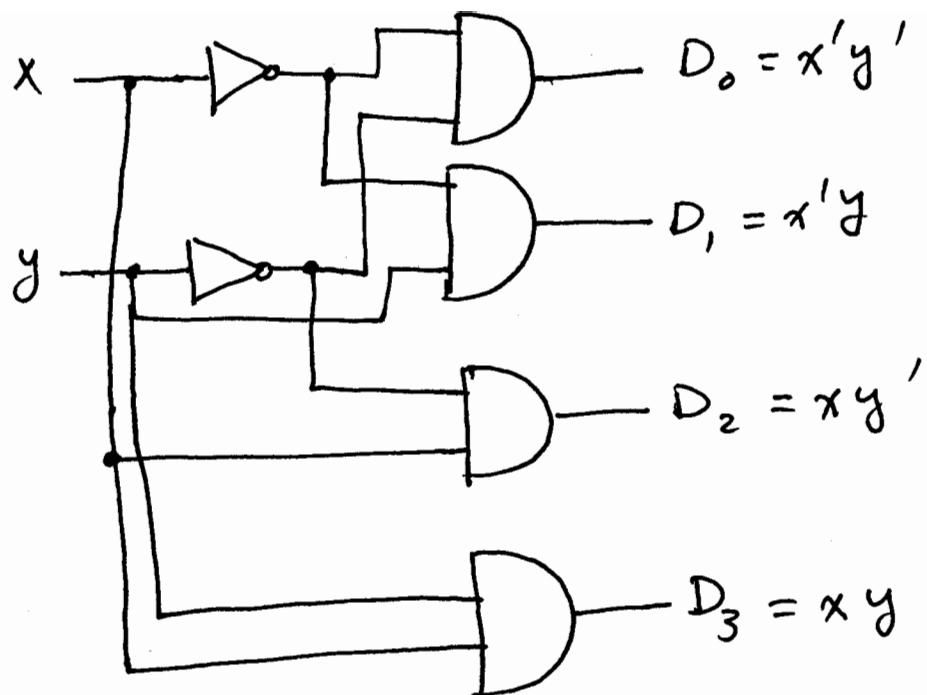
We can add an enable bit to the decoder. This input goes to all ANDs and lets the decoder to output the minterms only when it is equal to one. When enable bit is zero the output is all 0.
