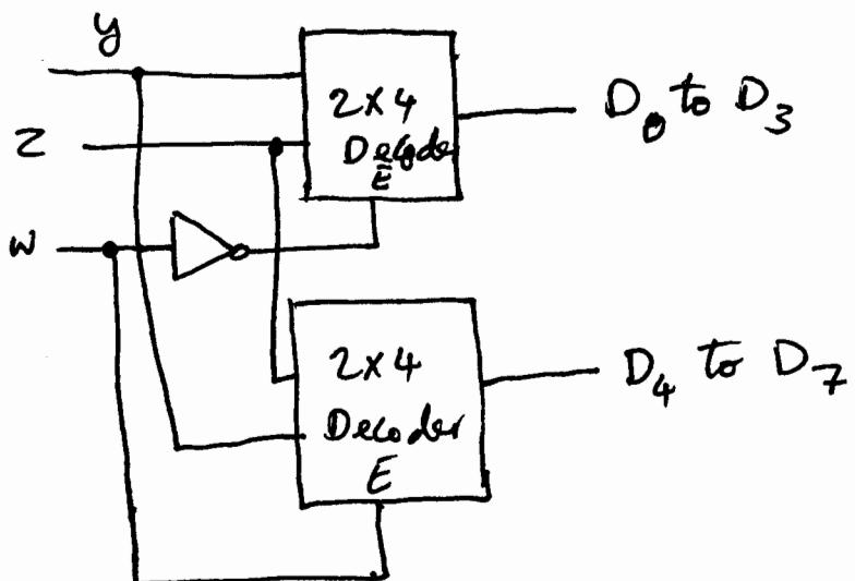
When  $W=0$  the first (top one) decoder is enabled and  $D_0$  to  $D_3$  represent  $w'x'y'$ ,  $w'x'y$ ,  $w'x'y'$  and  $w'xy$ .
