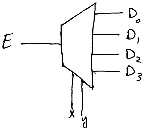
The demultiplexer is like a switch controlled by x and y.
