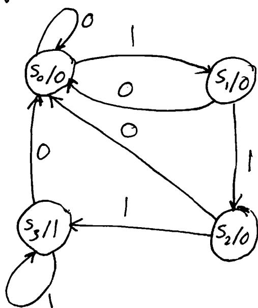
Drawing the above state diagram completes the first step in the design. It is clear that the number of states cannot be reduced.
