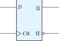
• A falling (negative) edge triggered D-flip-flop is represented by the symbol:
