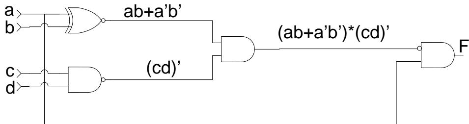
$$F = \overline{(\bar{a}b + \bar{a}\bar{b})\bar{c}\bar{d}} + a = (\bar{a}b + a\bar{b}) + \bar{c}\bar{d} + a = \bar{a}b + \cancel{a}\bar{b} + cd + a = \bar{a}b + cd + a = a + b + cd$$
