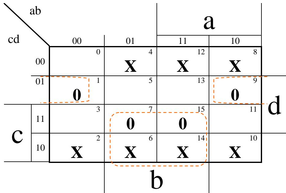
$$F = (b + c + \bar{d})(\bar{b} + \bar{c})$$
