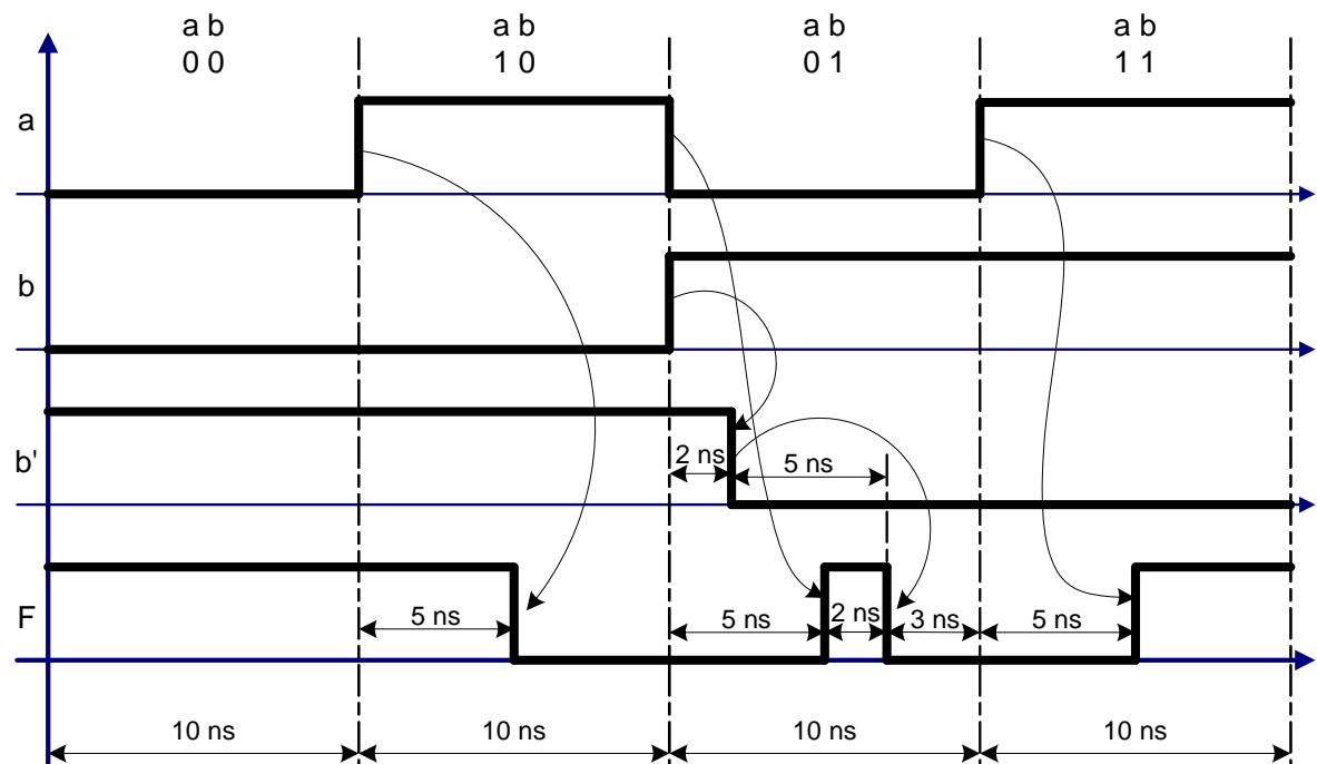
Edges that cause change in the output are shown with an arrow after delay of going through the gate.
