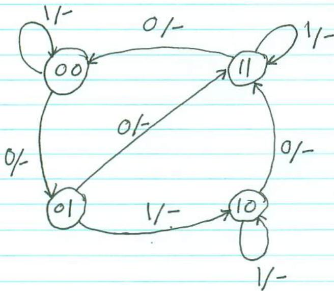
The sign - after / signifies the fact that this circuit does not produce any output.
