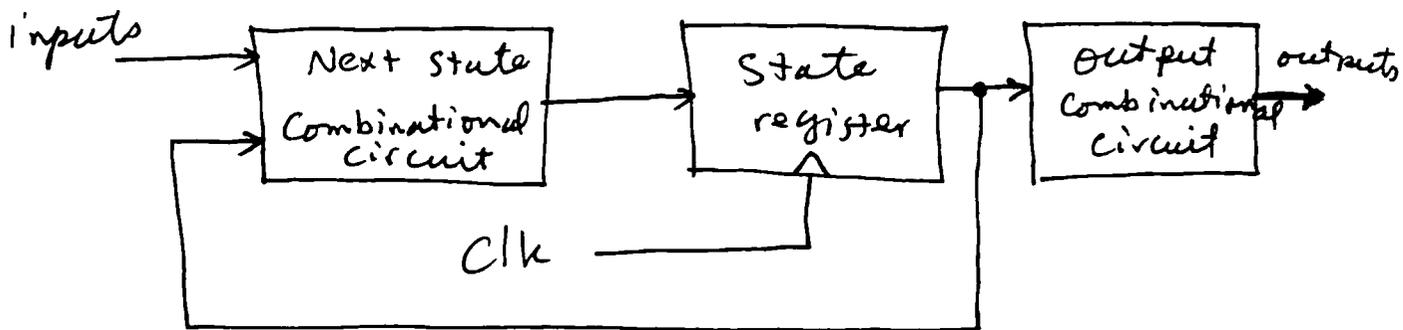
Another type of sequential circuit is a Mealy Machine. In a Mealy Machine, the output is formed by combining the present state and the present input:
