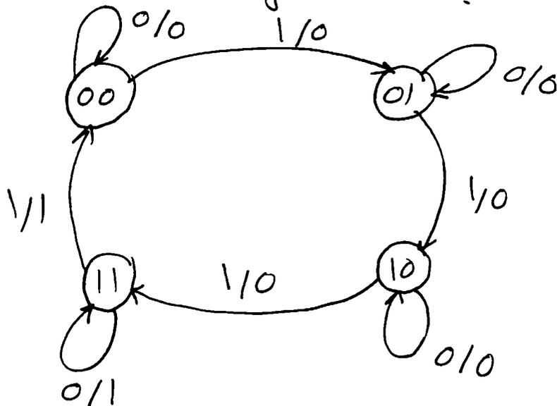
Note that in this state diagram, the output to an input is the same whether this input is 1 or 0. It only depends on the state where the FSM has been
