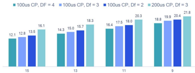
Fig. 13. System-level SNRs for car-mounted receivers in LPLT settings under the 50/1 ITU-R P.1546-5 channel model with small scale fading.
