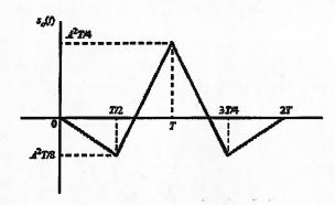
(c) The peak value of the filter output is equal to  $A^2T/4$ , occurring at t=T.
