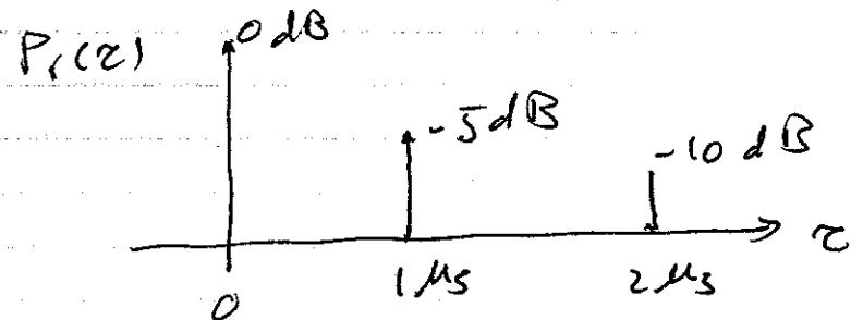
A mobile transmits at a rate of 500 kbps using QPSK with a raised cosine filter with roll-off factor of  $\alpha=0.5$  over this channel.
